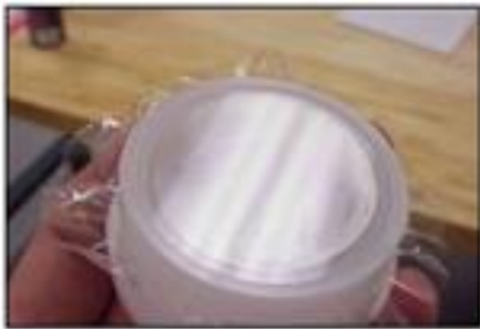
Correctly prepared sample cup – CAN USE
