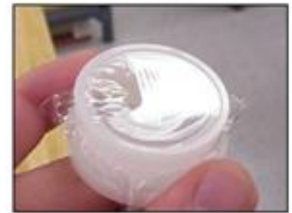
Incorrectly prepared sample cups – CANNOT USE
