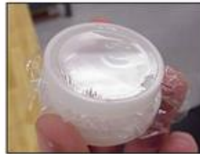
Incorrectly prepared sample cups – CANNOT USE
