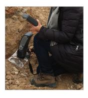
Large samples like long drill cores, pit walls, and chunks of material can be easily screened without the need to remove a sample.
