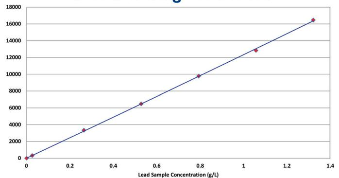
Sindie uses a weighted least squares regression in low range which is extremely linear and easy to set up. Typical correlation (R value) is expected to be on the order of 0.999 or better.
